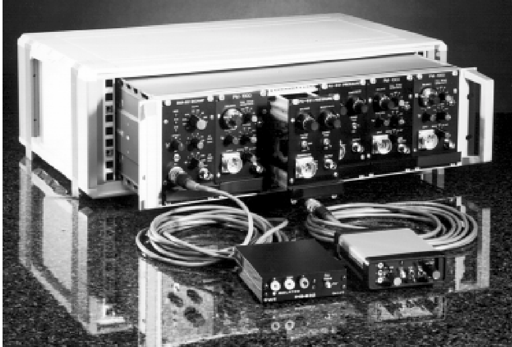
Above: Desktop enclosure (DTE-1000) housing CC-1000 amplifier cage. Six plug-in amplifiers fully populate the CC-1000.
